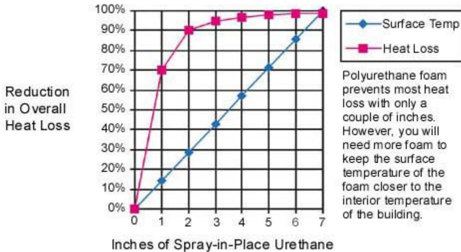
*This graph illustrates the reduction in heat loss from a building when it is insulated with various thicknesses of spray-in-place urethane foam. Note: the insulation benefit tops off very quickly above three inches. The*
